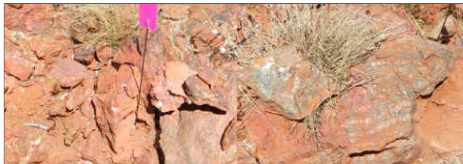
Figure 3-40: Weathered haematitic, siliceous rock with boxworks (left) and banded quartz green mica-limonite rock (right)
