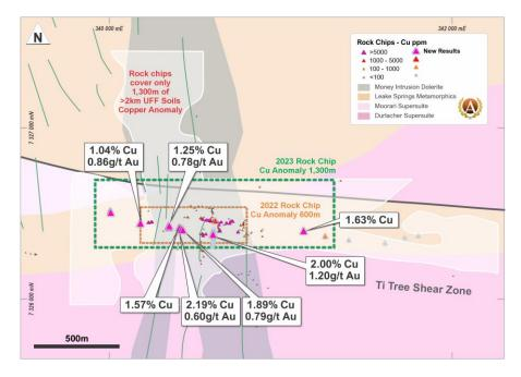
Figure 3. Detailed Map of Copper Ridge showing extensions of mineralisation
