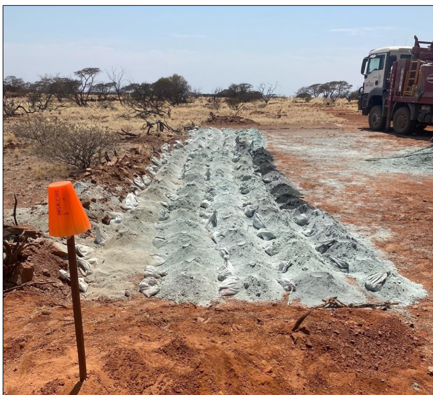
Figure 2. Hole MSRC012 – showing black RC piles containing copper sulphides.
